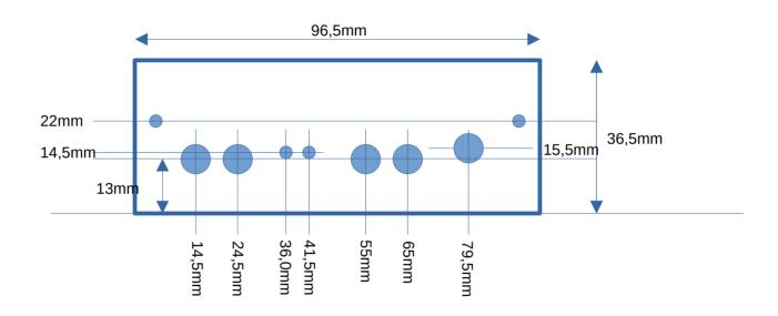
LED holes 3mm, all other holes 7mm diameter. View from inside (backside) of front panel. Drill from this side.
